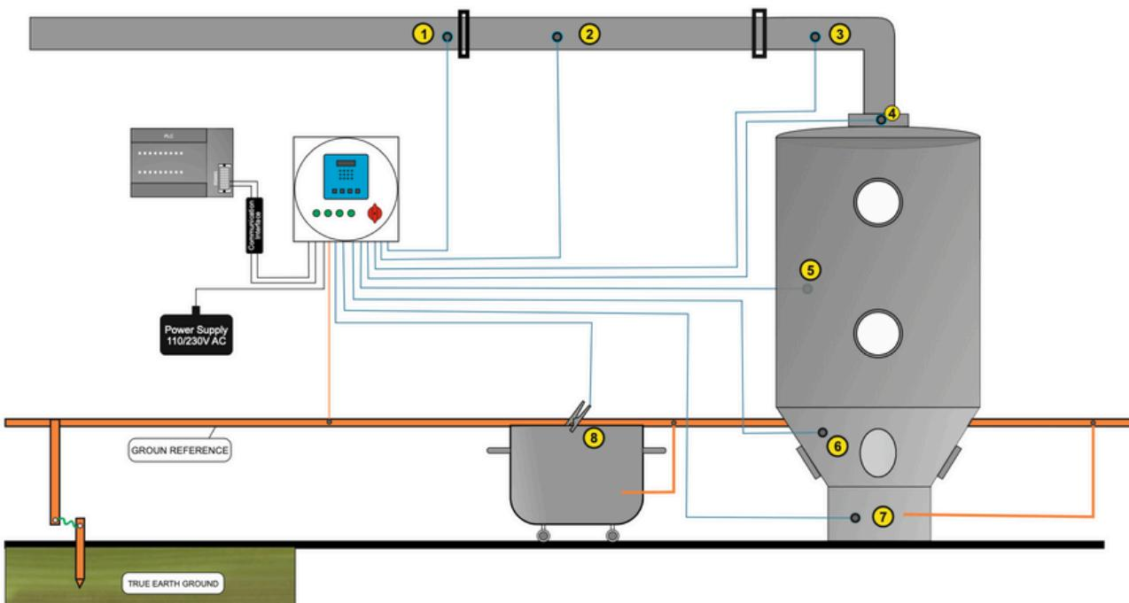
In this setup, EMS monitors grounding for a fluid bed dryer system. A marshalling enclosure distributes signals from seven channels to permanent grounding points installed on ducts, hoppers, and processing sections. Eight channels feed permanent grounding points on interconnected equipment, with all channels grouped to control powder flow only when proper grounding is confirmed. The system is connected to the PLC via Modbus communication to monitor the status remotely.
